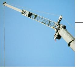
**Tip height** Maximum tip height of 47,0 m (154 ft) with 13,7 m (45 ft) telescopic extension.
