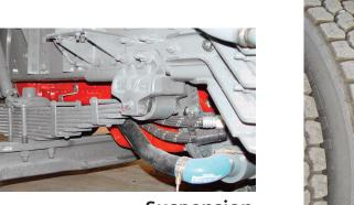
**Suspension** Spring front suspension with air ride rear suspension provides a comfortable ride at 105 km/h (65 mph).
