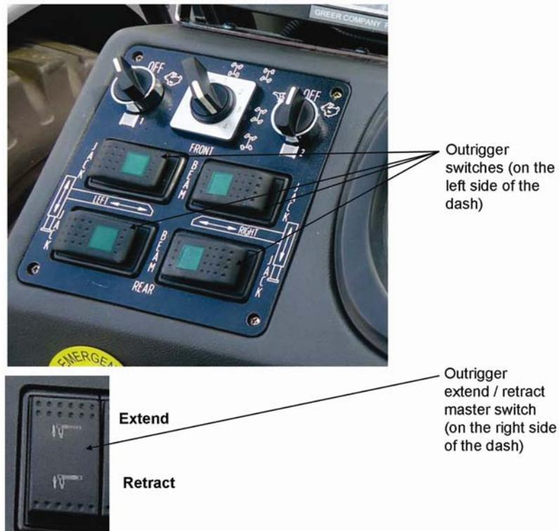
Figure 07 – 4 Outrigger Switches
